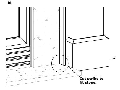
If using a hearth that fits between the leg opening, cut the scribe to allow for stone height between the legs. Place the scribe molding as shown above, positioning it so that it just contacts the noncombustible surround. Be careful not to hit the facing material when nailing the scribe in place. No cutting is needed if hearth exceeds mantel legs.
