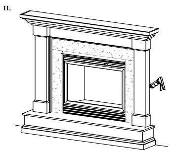
Caulk the mantel to the wall all the way around, using a caulk that matches your mantel color. This will eliminate any remaining gap between mantel and wall.
