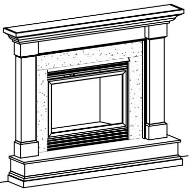
Kenwood mantel with optional base. Note: Using the base will raise the fireplace by 9-1/4" above finished floor level. All dimensional requirements of fireplace installation should be ajusted accordingly.
