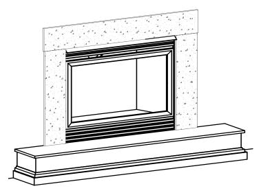
Install non-combustible facing material such marble, granite, tile using High Temp. adhesive.
