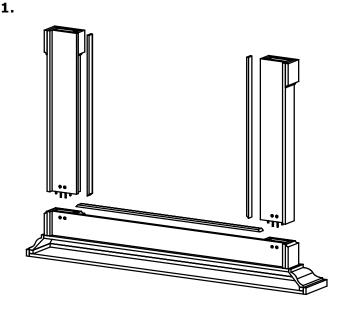
Position the top assembly (a) of mantel upside down on a flat, clean, non-abrasive surface. If scribe molding (d) was shipped attached to the leg and breast board, remove it before beginning assembly. Pry gently from the rear with a flat screwdriver.
