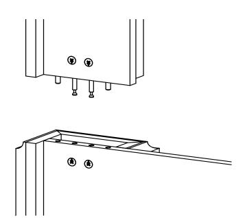
Attach one leg assembly (B) to breastboard assembly by inserting dowels and cam pin into matching holes on ends of breastboard. Before inserting, make sure that the arrow on the cam in breastboard points toward the edge of board as shown in inset. (Dowels and cam pins are shipped pre-inserted in the end of the leg assembly.)
